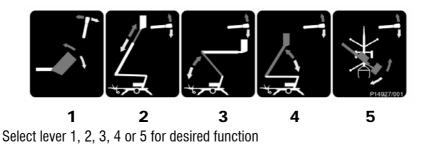
1Operates Platform Lev.FWD for forwardBACK for back2Operates TelescopeUP for outDOWN for in.3Operates Lower BoomUP for upDOWN for down4Operates Upper BoomUP for upDOWN for down5Operates SwingUP for rightDOWN for left
